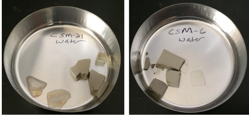
Figure 2: Degradation of CSM-21 (Hi SO4) and CSM-6 (Ave) after Water-Saturation.
