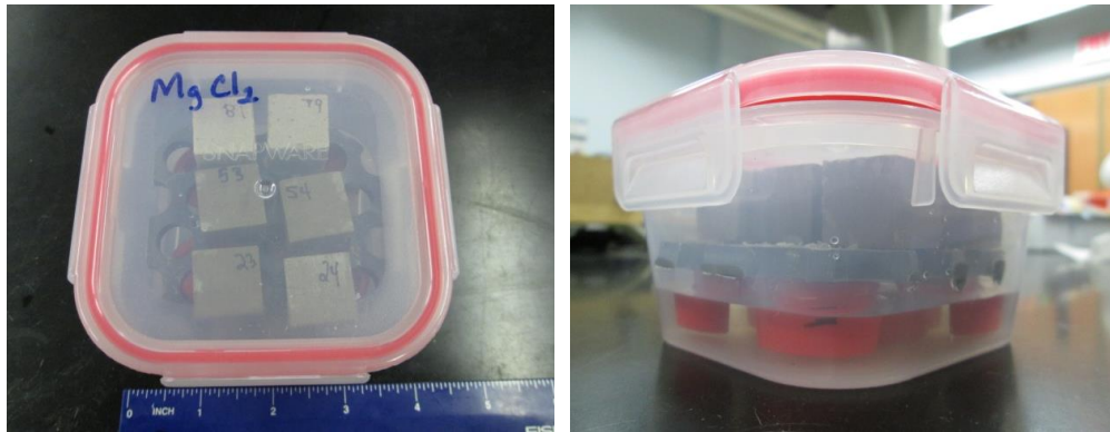
Figure 5: Storage of CSM Samples in a Controlled Environment at 33% RH.
